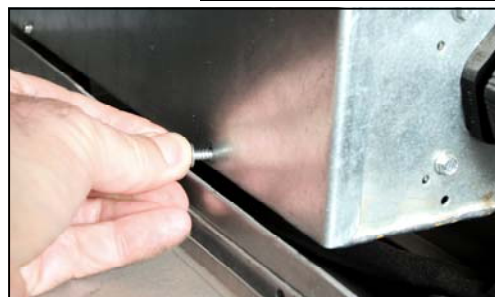
Figure 1: If the failed actuator is over a side-mounted contactor box, remove the rearmost screw from the top of the contactor box. The lower position of the new actuator requires a lower position for the box. The screw is inaccessible after the box is lowered.
