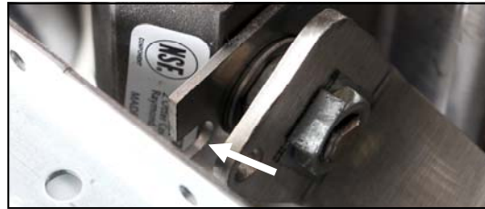
Figure 5: Use a pin to align the valve bracket with its alignment hole, ensuring the valve is fully closed. See arrow.
